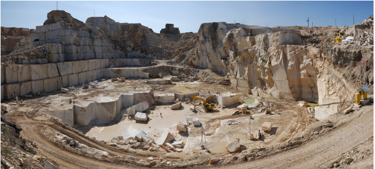
Fig. 1. Iscehisar, Afyonkarahisar. Overview of the Bacakale district (2008). On the left side the northern limit with modern fronts cut with diamond wire, on the right side the southern roman quarry front (photo: Turgut Tarhan)
