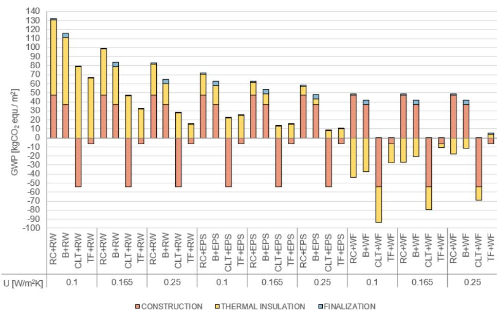
**Figure 2.** Global warming potential of external wall components
