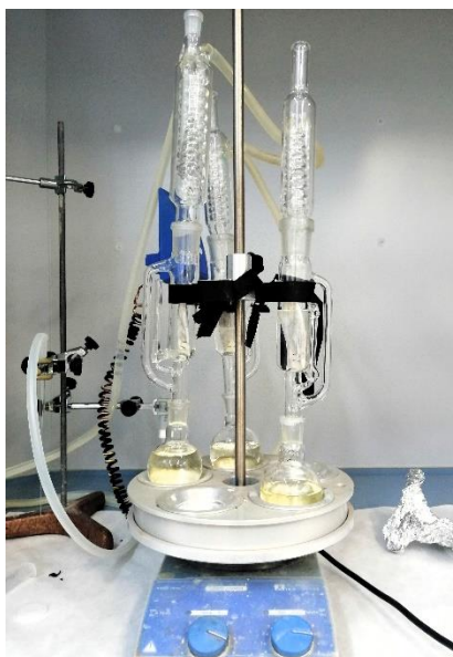
Figure 16. Soxhlet extraction of the samples.
