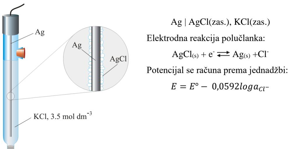
**Slika 8.** Shematski prikaz  $\text{Ag}/\text{AgCl}$  elektrode<sup>17</sup>
