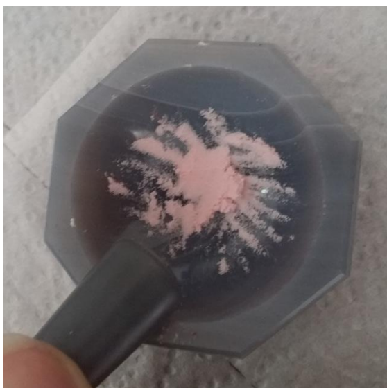
Figure 6 Adding KBr to the sample and homogenizing material for the pellet
