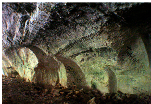
Fig. 8. Traces of rock exploitation in the gallery quarry on Sutvara Island (photo: M. Parica)
