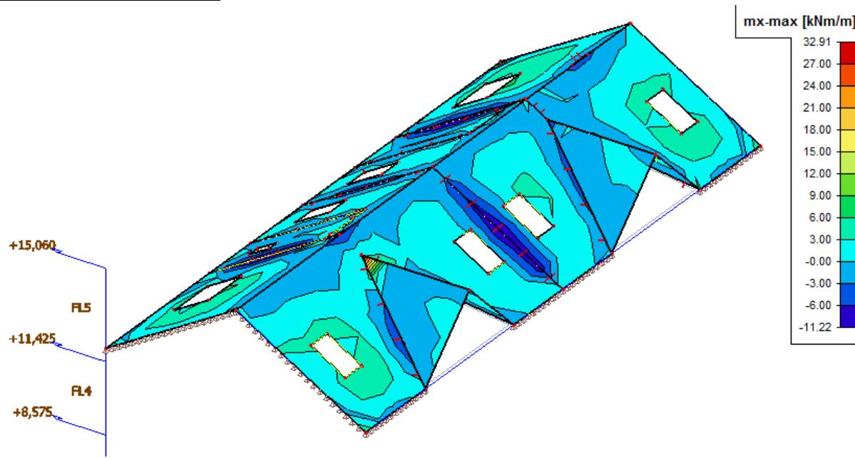
Slika 38: Prikaz momenata savijanja  $M_x$ (kNm/m')
