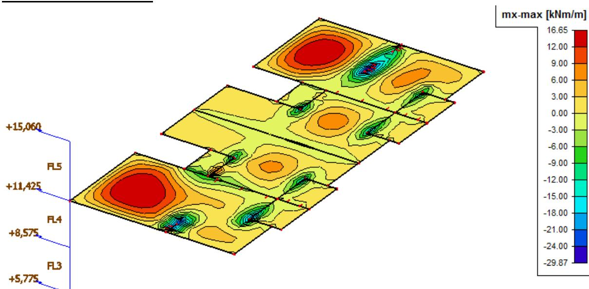
Slika 30: Prikaz momenata savijanja  $M_x$ (kNm/m')
