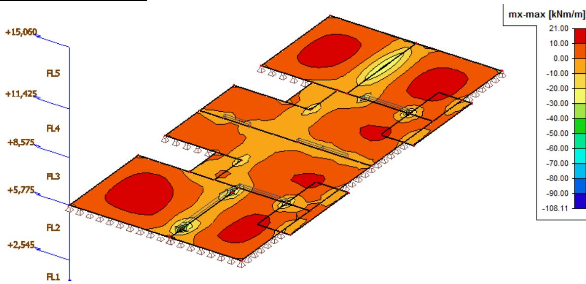
Slika 26: Prikaz momenata savijanja  $M_x$ (kNm/m<sup>2</sup>)
