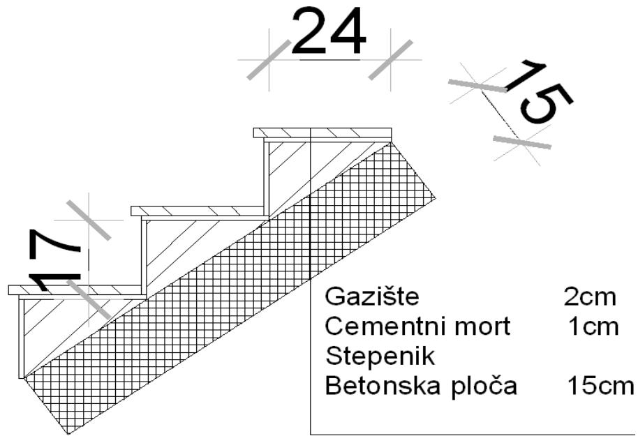
$$\operatorname{tg}\alpha = \frac{v_{st}}{v_{st}} = \frac{17}{24} = 0,7083 ; \alpha = 35,31^0$$
