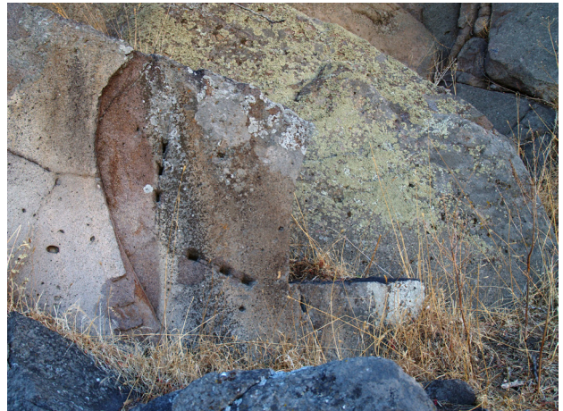
Fig. 5. Wedge-holes on a vertical rock surface before splitting in the south-eastern quarry in Larisa West (photo: © Archive of Larisa)
