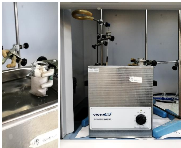
Figure 15. Ultrasound assisted extraction of the lichen.
