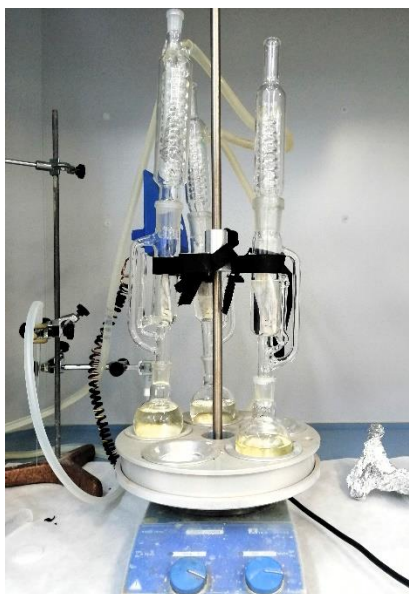
Figure 16. Soxhlet extraction of the samples.
